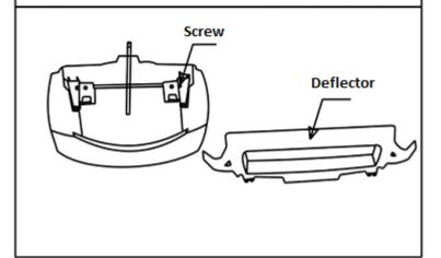
Position the front air baffle, fix the noses on the provided lots and screw them firmly.
