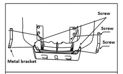
Bottom up the main body of the vehicle with the underside and connect the front bumper. Position the metal brackets and connect the front bumper with the main body so that the brackets are screwed both on the main body and the front bumper.
