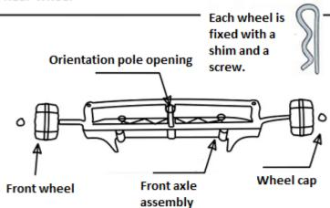
FIXING THE FRONT AXLE ASSEMBLY
