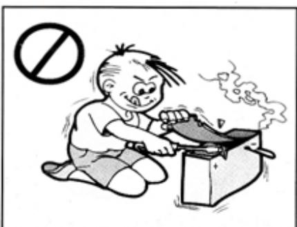
**NEVER OPEN THE BATTERIES** THEY INCLUDE LEAD AND CORROSIVE ACID. WHEN THERE IS A SKIN CONTACT OR SWALLOW, THEY MAY LEAD TO CORROSION AND SERIOUS INJURIES.
