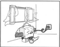
DURING THE CHARGING PROCESS, EXPLOSIVE GASES MAY COME INTO EXISTENCE. CHARGE THE BATTERIES ONLY IN A WELL AIR CONDITIONED ROOM AND KEEP THEM AWAY FROM INFLAMMABLE MATERIALS.
