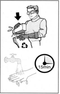
IF THE BATTERY LEAKS, AVOID SKIN AND EYE CONTACT WITH THE LIQUID OF THE BATTERY AND PUT THE BATTERY IN A PLASTIC BAG. PLEASE READ THE INSTRUCTIONS IN THE OPERATION MANUAL IN ORDER TO LEARN HOW TO DISPOSE THE BATTERY.
