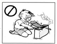
NEVER OPEN THE BATTERIESS THEY INCLUDE LEAD AND CORROSIVE ACID. WHEN THERE IS A SKIN CONTACT OR SWALLOW, THEY MAY LEAD TO CORROSION AND SERIOUS INJURIES.
