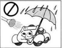
THE VEHICLE, CABLE CONNECTIONS, MOTOR AND BATTERIES MUST BE KEPT AWAY FROM WATER. DO NOT WASH THE VEHICLE WITH A WATER HOSE.
